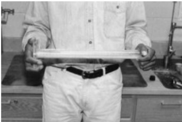
Figure 4 —Using Hand Method of Shaking
