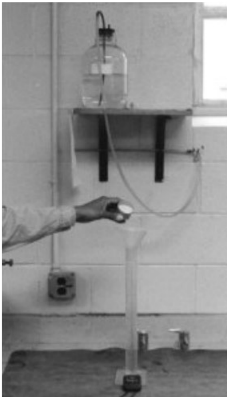
Figure 3 —Transfer of Sample from Measuring Tin to Cylinder
