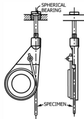
FIG. A4.2 Snubbing-type Gripping Device
