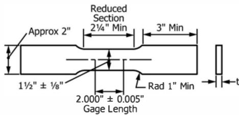
NOTE 1—The dimension *t* is the thickness of the test specimen as provided for in the applicable material specifications.
