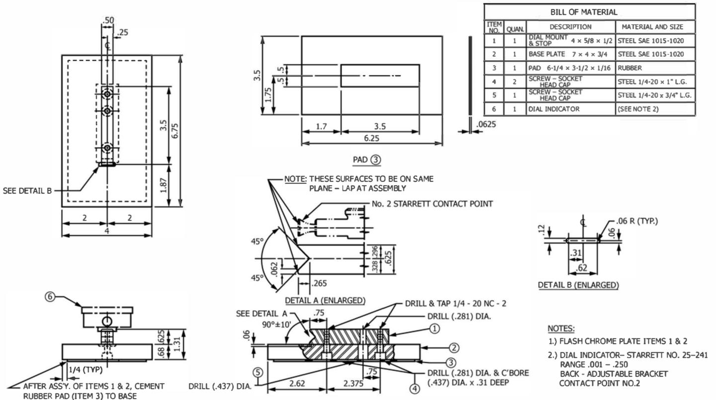
FIG. 17 Assembly and Details for Lateral Expansion Gauge
