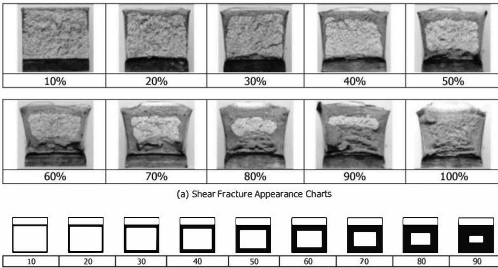
FIG. 14 Fracture Appearance Charts and Percent Shear Fracture Comparator
