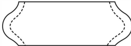
**FIG. A2.10 Crush Test Specimen**
