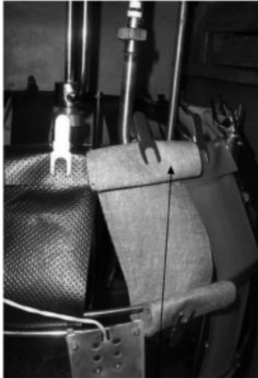
FIG. 3 Roller Grip Specimen in Weathering Device
